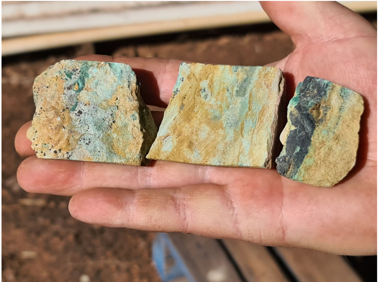
Figure 1: drill core showing the cross-cutting nature of the copper mineralisation
